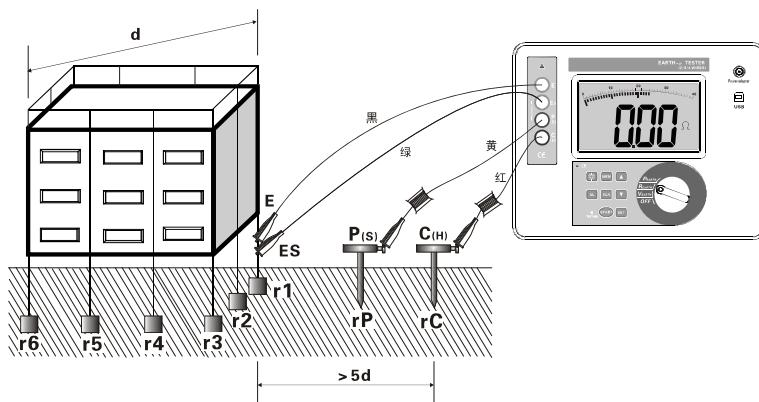
$R=r_1//r_2//r_3//r_4//r_5//r_6//\dots//r_n$  ( $r_1\dots r_n$  都是独立接地点)
